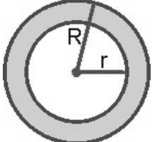
$$A(\text{corona}) = \pi R^2 - \pi r^2 \xrightarrow{\text{sacando factor común } \pi} \boxed{A(\text{corona}) = \pi(R^2 - r^2)}$$
