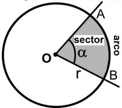
$360^\circ \rightarrow 2\pi r \Rightarrow \widehat{AB} = \frac{2\pi r \cdot \alpha}{360^\circ} \Rightarrow \boxed{\widehat{AB} = \frac{\pi r \alpha}{180^\circ}}$ $360^\circ \rightarrow \pi r^2 \Rightarrow S = \frac{\pi r^2 \cdot \alpha}{360^\circ}$ $P = r + r + \widehat{AB} = \boxed{2r + \frac{\pi \cdot r \cdot \alpha}{180^\circ}}$ |
