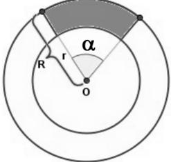
$$360^\circ \rightarrow A(\text{corona}) = \pi(R^2 - r^2) \Rightarrow \boxed{T = \frac{\pi(R^2 - r^2) \cdot \alpha}{360^\circ}}$$
